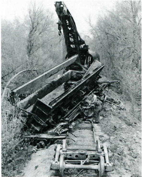
When an air dump car tipped over near Seeley Creek, Mid-Continent put it back on the track May 8 in the historic way, using a steam-powered wrecker. Bill Raia was at the controls of ex-MP x105. Among those helping were Mike Raia; Wally Johnson, Soo Line wrecking foreman; Skip Lichter; Stan Nordeng; Mark Rosemont; Jeff Bloohm; Paul Young; and Bob Welke. Photo by Paul Swanson
