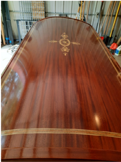
A pair of the original upper berths after they have been restored and following fresh coats of stain and varnish
