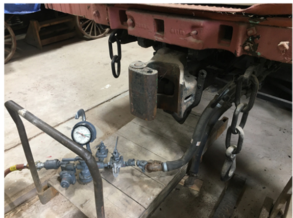
View of the air brakes being tested on the DULUTH
