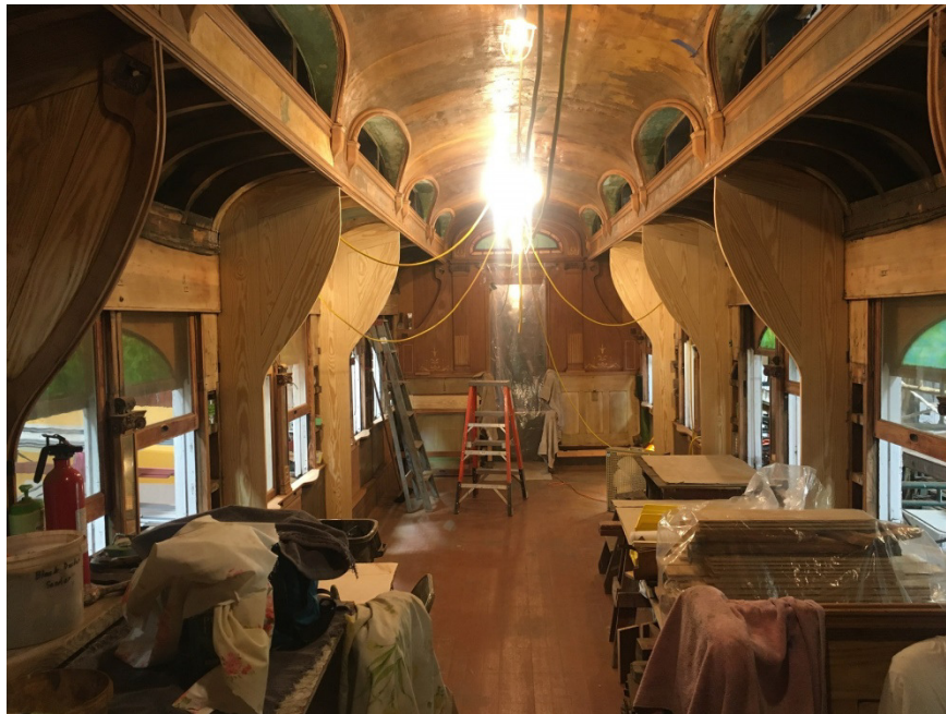
View of the sleeping compartment showing the woodwork that has been stripped during 2021
