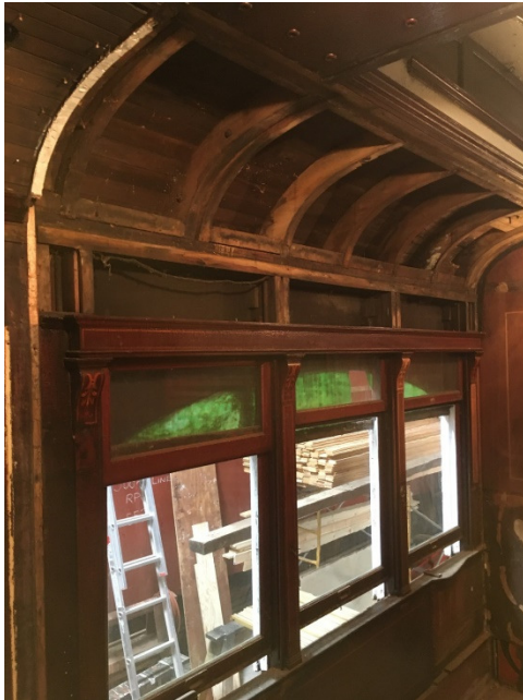
The east wall of the smoking room showing the headliner and upper wall panel removed
