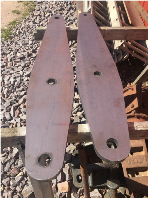
Two of the new brake cylinder levers that were made. The steel levers are 1 inch thick and 36 inches long
