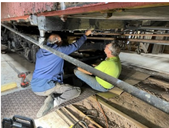
Volunteers installing some of the hand brake brackets
