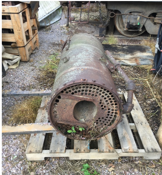
Baker Car Heater acquired for use in the DULUTH. Awaiting restoration
