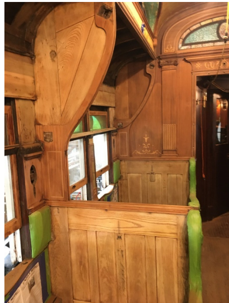
Interior woodwork in the process of being stripped inside the DULUTH
