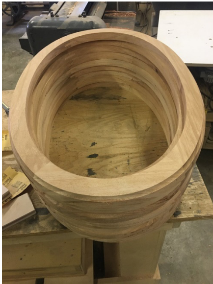
New replica oval window frames (L) and new lower sash window frames (R) made this past year for the DULUTH
