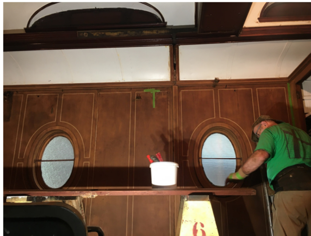
The west wall of the car across from the smoking room showing the stripping in process
