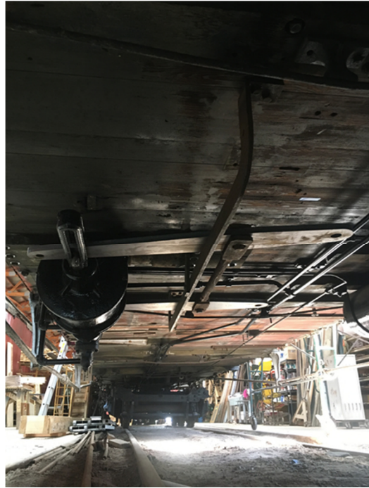
The bottom side of the DULUTH showing the air cylinder with the new levers, rods and hangers installed
