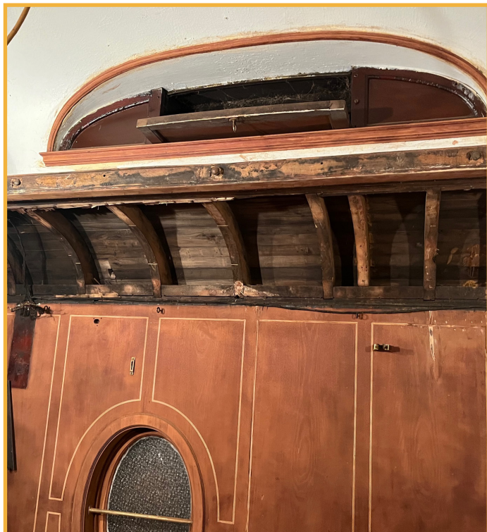
The deteriorated headliner in the process of being removed from the lower roof across from the smoking room.
