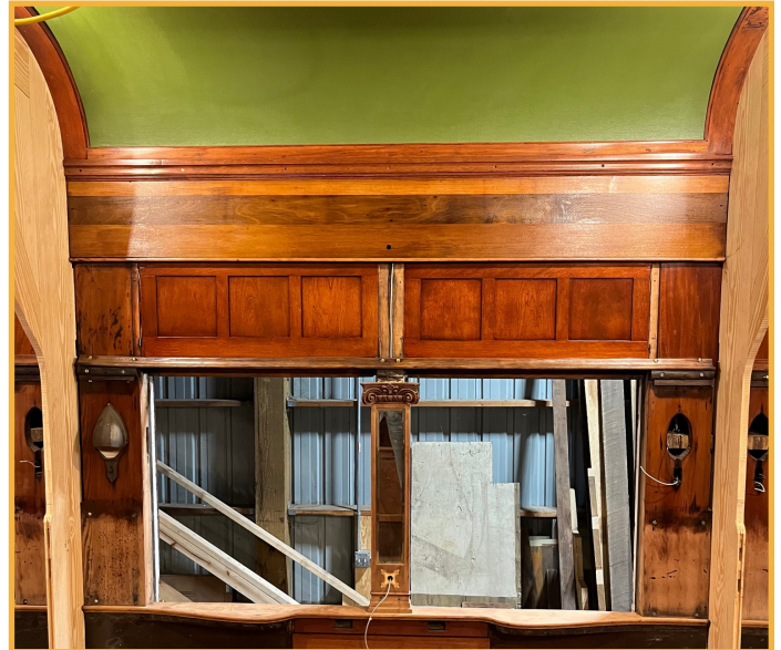
The berth side walls with the headliners and wood blinds installed. One coat of finish was applied on all of the woodwork.
