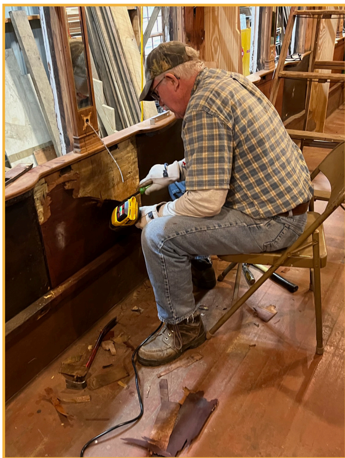
Volunteers removing deteriorated veneer pieces from below the windows in the sleeping compartment.
