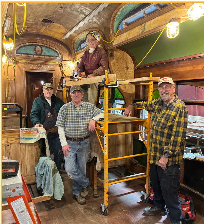
The volunteer crew working on cutting and removing the deteriorated portion of the upper clerestory ceiling.
