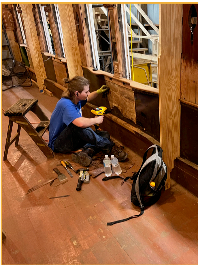
Volunteers removing deteriorated veneer pieces from below the windows in the sleeping compartment.
