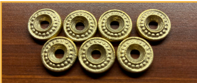
Newly cast brass grommets for the shade boxes.
