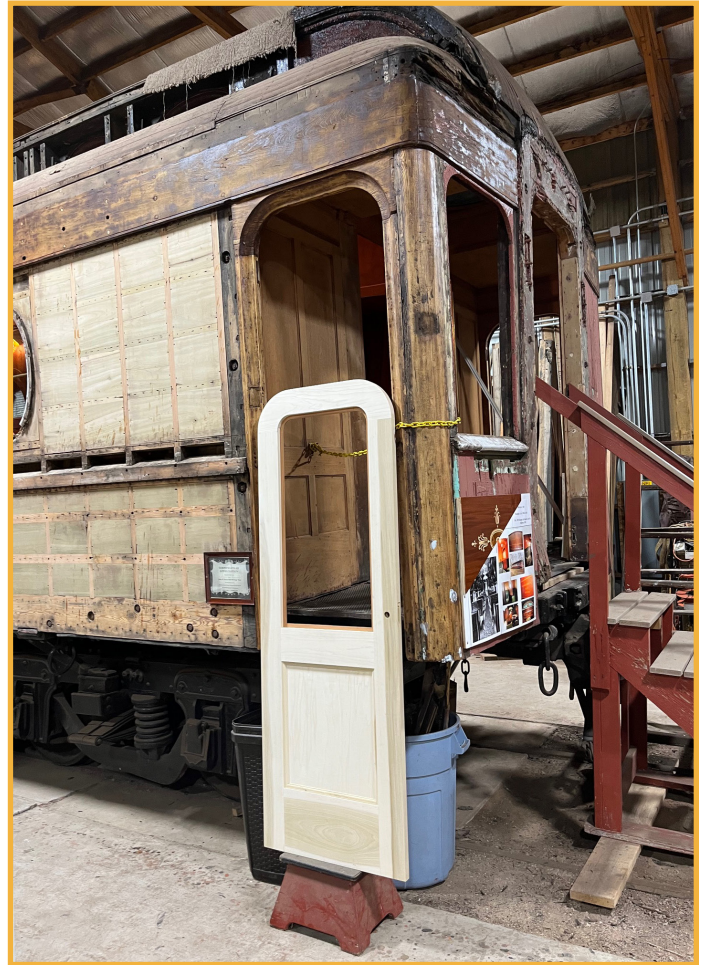
Four new vestibule doors were made to match the original design that featured a larger window size. Left photo: 1918 era replacement vestibule door (L) next to the reproduced original design door. (R)
