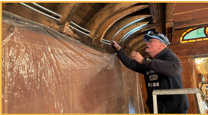
A volunteer installing flexible metallic conduit for the sleeping compartment annunciator wires.
