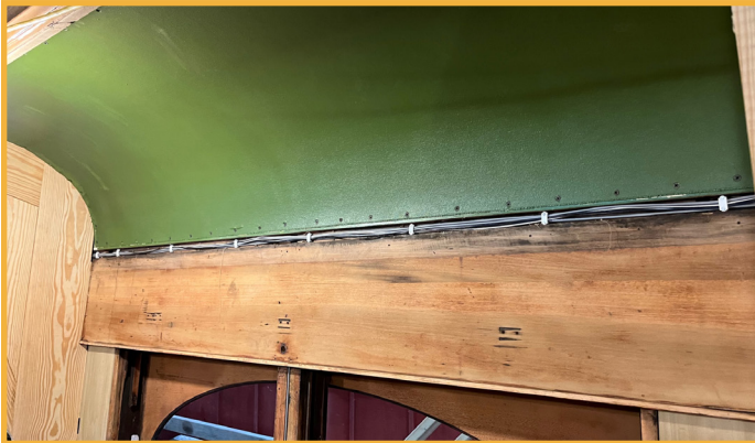
Newly installed electrical and annunciator wiring routed below the headliner panels in the sleeping compartment.
