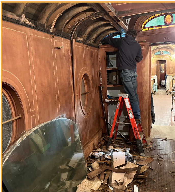
The deteriorated headliner in the process of being removed from the lower roof across from the smoking room.
