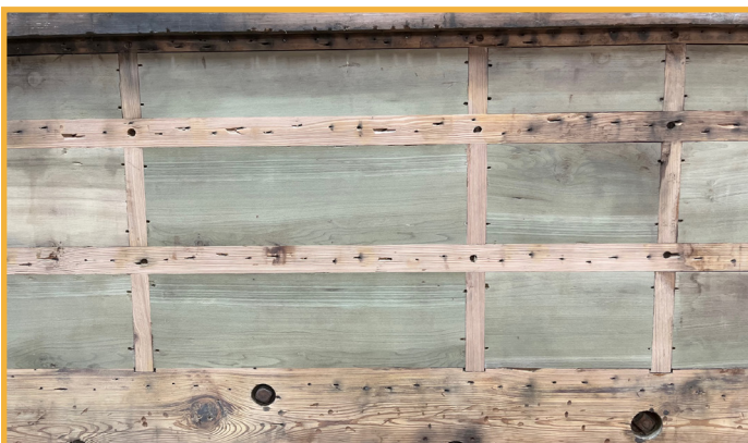
The lower exterior framing after being completely sanded to remove all of the old glue from the car.
