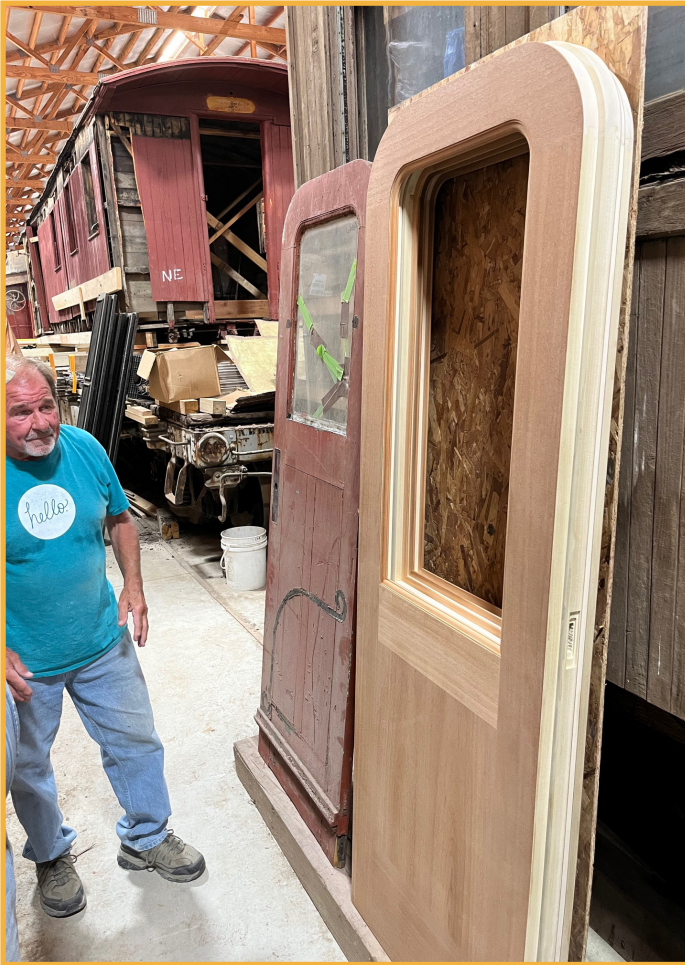
Four new vestibule doors were made to match the original design that featured a larger window size. Left photo: 1918 era replacement vestibule door (L) next to the reproduced original design door. (R)
