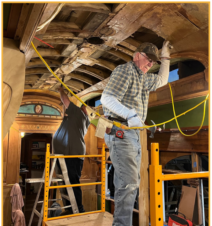
The volunteer crew working on cutting and removing the deteriorated portion of the upper clerestory ceiling.
